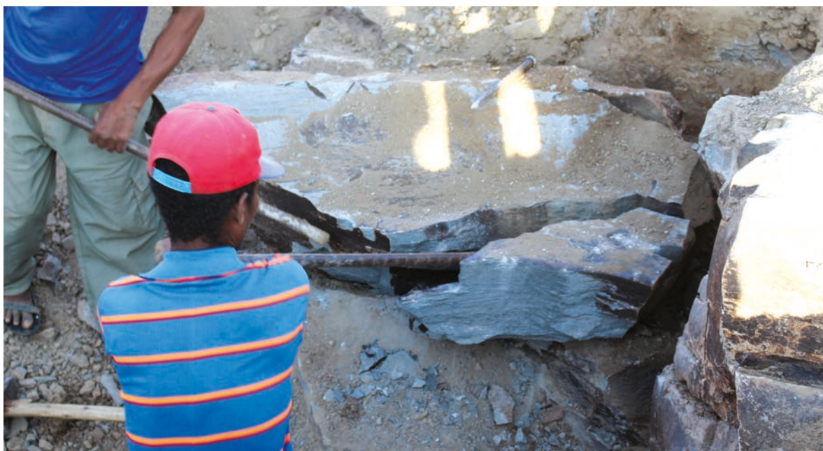
Figure 12. Miners breaking rock without PPE, site 3.
